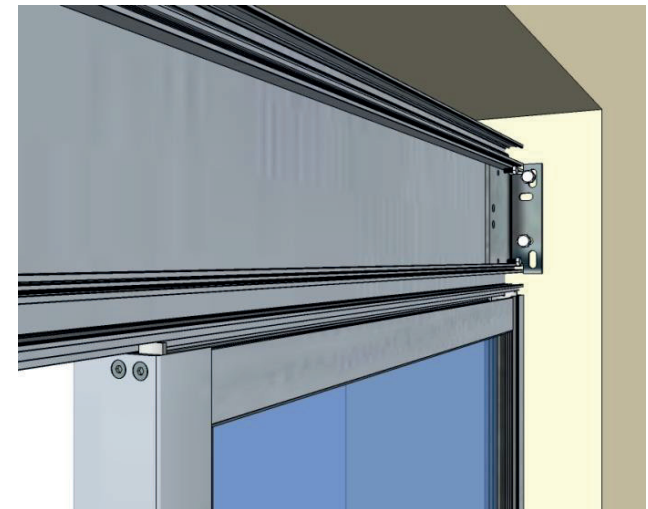
Wing lateral side fixing
